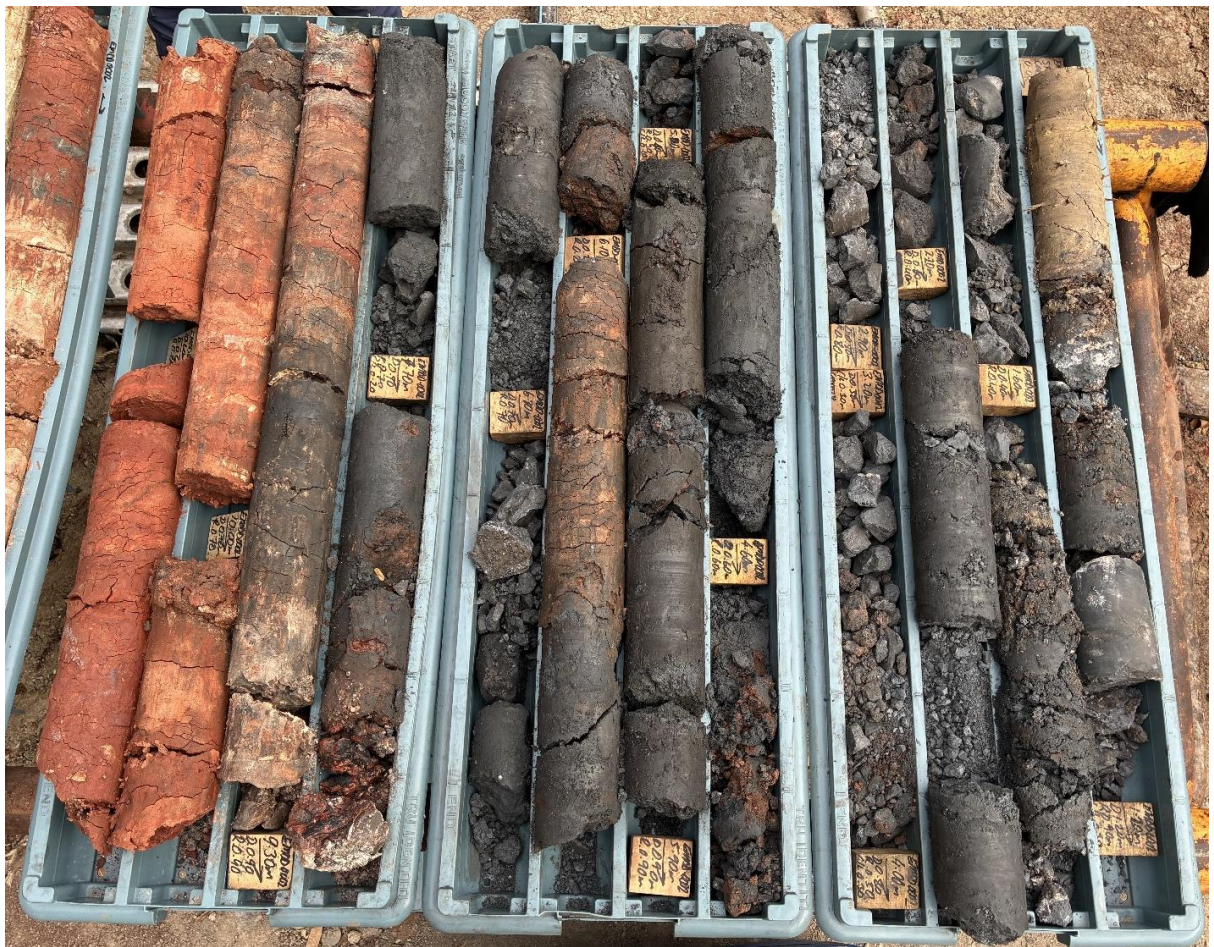
Figure 4: Tray 1 (right) to tray 3 (left) of EMDD002 showing the full intersection of PQ core with visual estimates presented in Table 3
