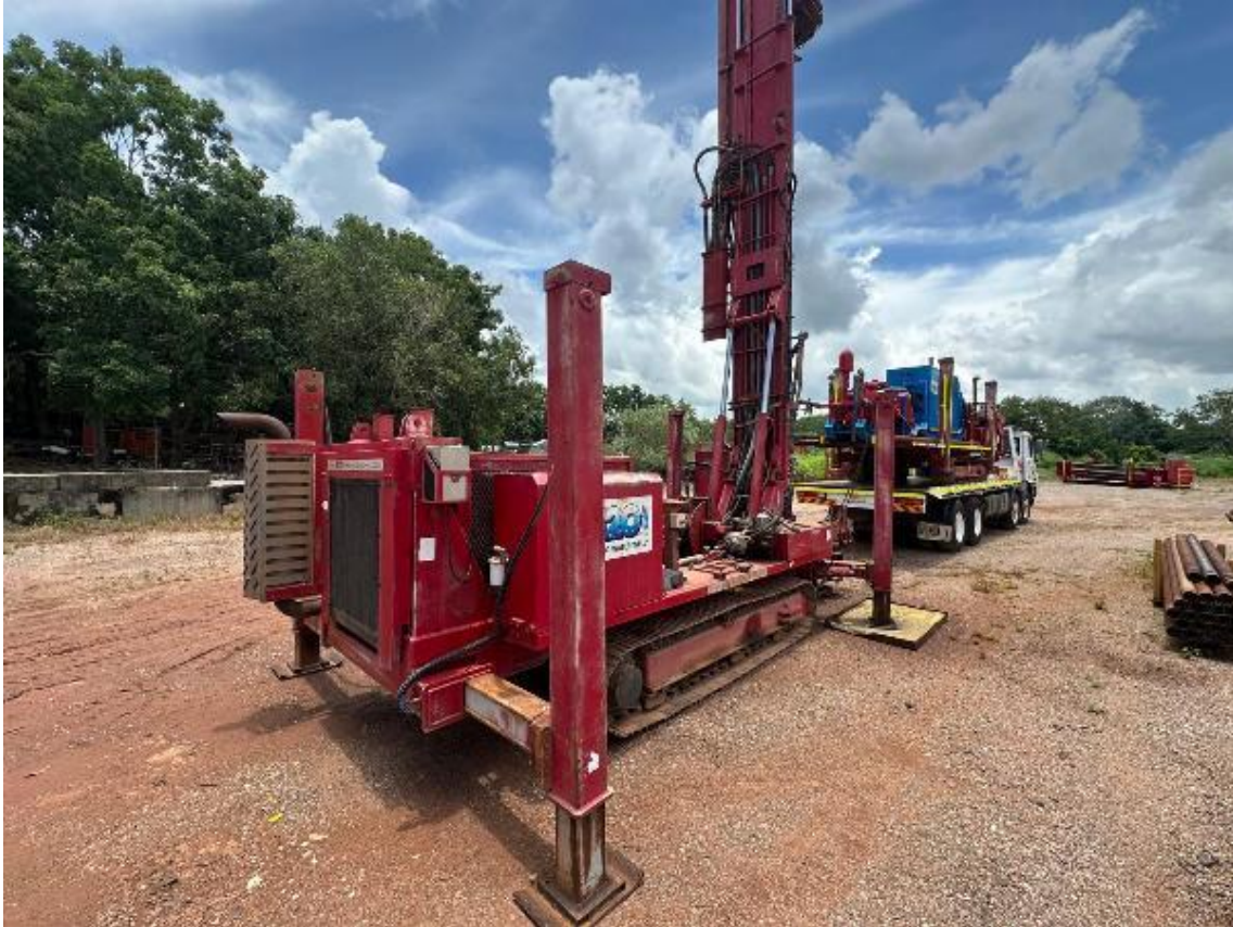
Figure 6: CoreSearch RC/DD rig with 1200 cfm of compressed air.
