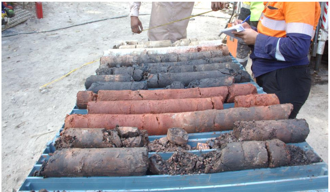
Figure 1: Secondary and detrital manganese in EMDD022. For visual estimates and visual estimates disclaimer please refer to Table 2. Assay results are expected in 6 weeks.
