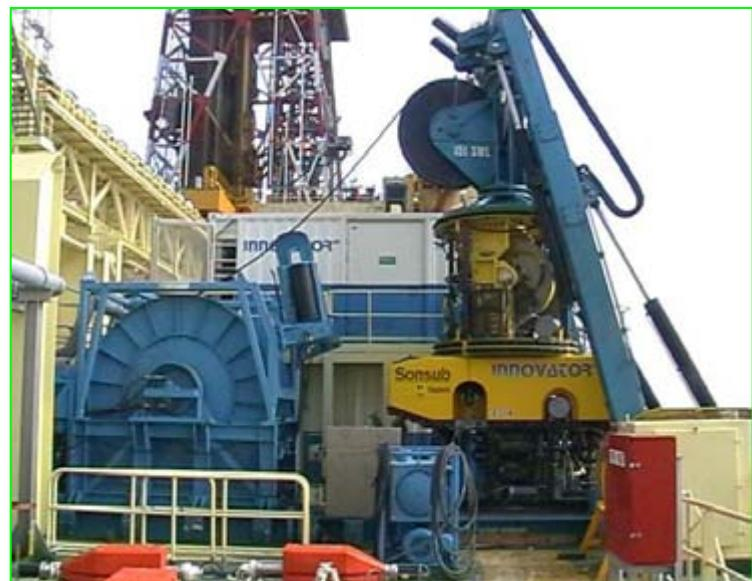
Remote Operated Vehicles (ROV) with cameras, used for viewing activities underwater
