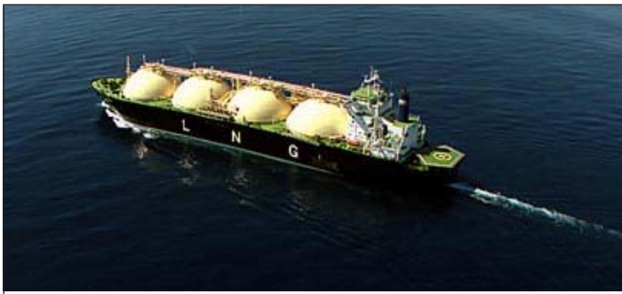
An LNG tanker, carrying its super cooled cargo to customers across the seas. A ship like this is usually about 300 meters (three football fields) long.
