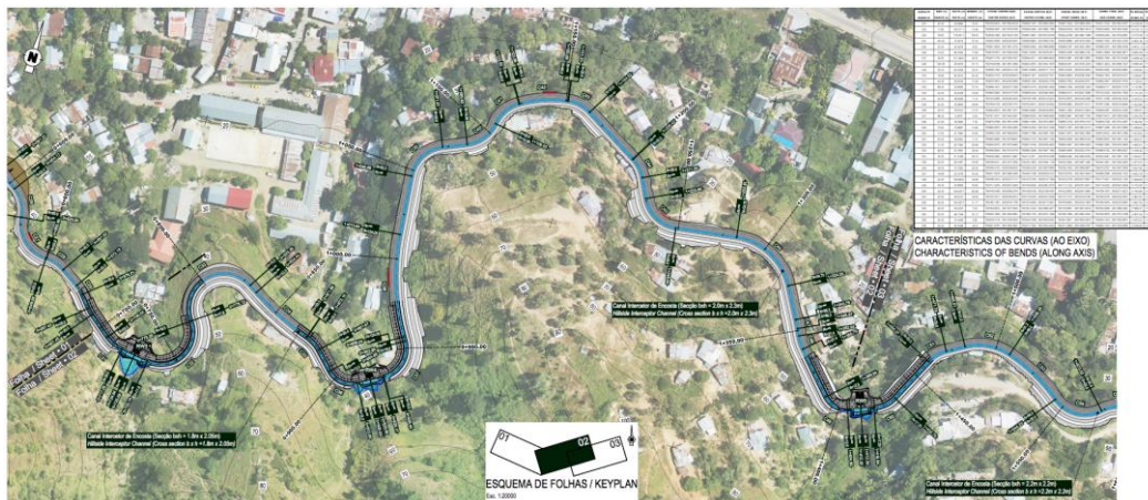
Figure 4 Mascarenhas Hillside Interceptor Channel Longitudinal Profile and Plan over Aerial Photograph - Section 3 (Source: AdP-TL, 2014)
