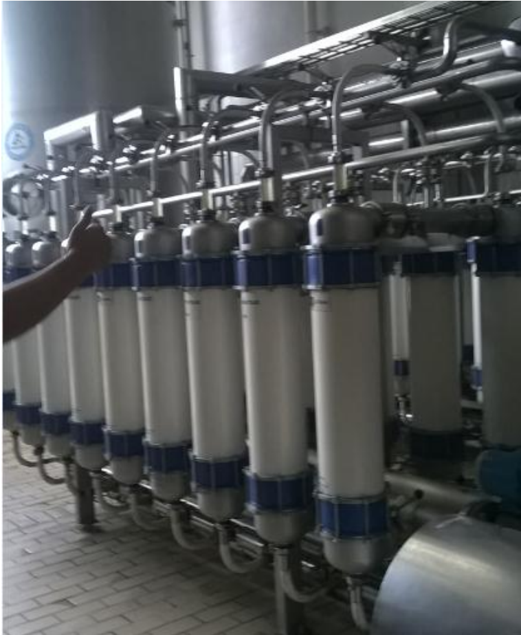
Figure 4.15 Micro-Filtration unit that Filter the Mature Beer (Courtesy of Heineken Indonesia)
