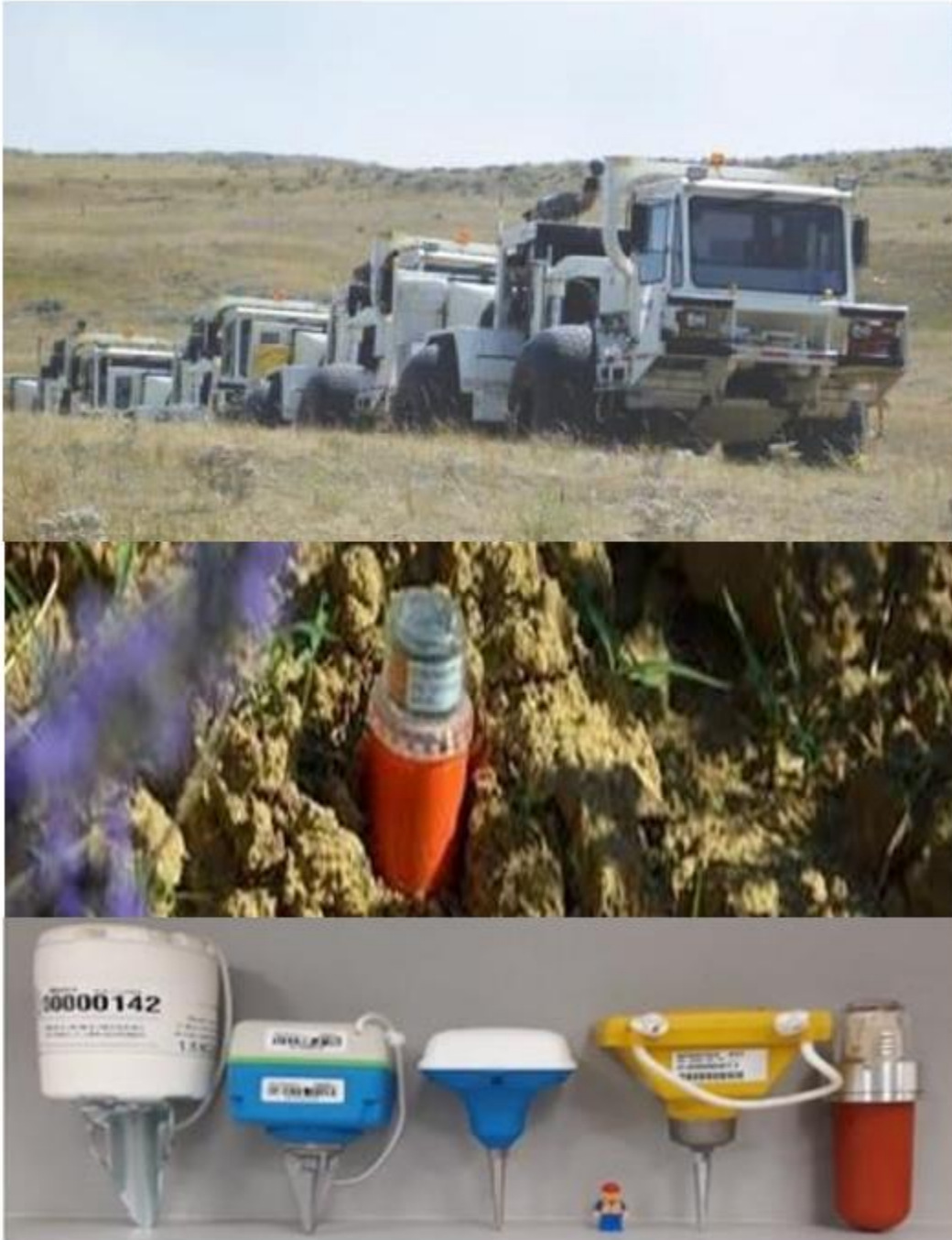
Figure 5. Vibroseis and Wireless Nodes (Source: Dawson Geophysical Web site)
