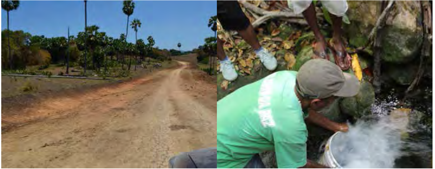
From left to right: Newly opened access road to the proposed area for Nova Beaço & Nova Knua's ; SAS Technician undertaking manual measurement of water flow rate at Ulu-Ira Spring
