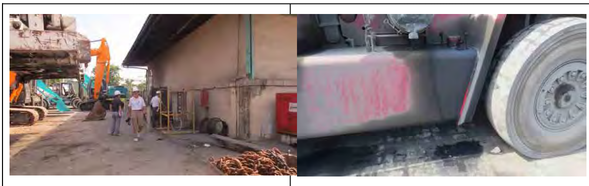
Figure 1.5-5 Oil Leak and Contamination in Workshop
