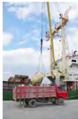
Figure 6.1-2 Quay-side Handling of Bag Cargo (cement)
