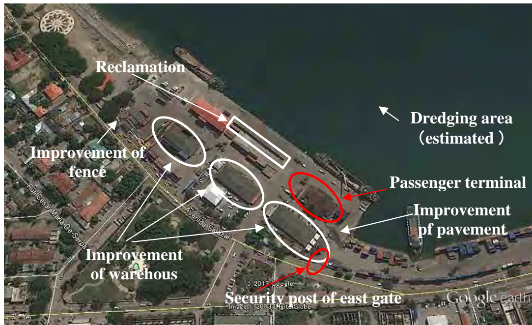
Figure 4.2-2 Location of Improvement Facility
