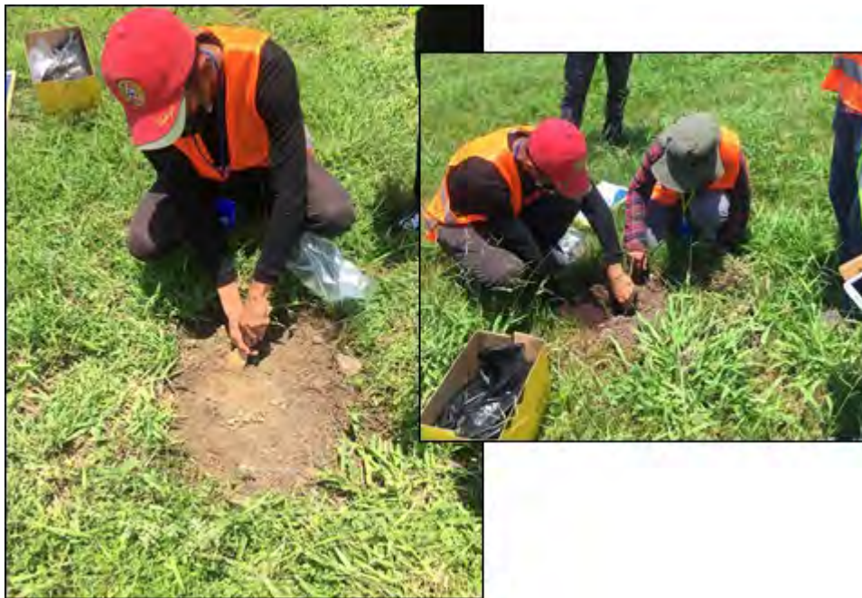
Figure 1.10 Soil sample collections in one of the locations inside PNLIA.
